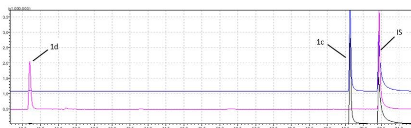
Figure S8: GC/MS chromatogram of conversions of 2-ethylbenzene-1,4-diol 1c . Black: with 8 mM ascorbic acid, pink: without ascorbic acid, blue: without enzyme, with 8 mM ascorbic acid. 10.7 min: 2-ethyl-1,4-benzoquinone 1d , 19.6 min: 2-ethylbenzene-1,4-diol 1c , 20.5 min: IS. Reactions were conducted in 50 mM sodium phosphate buffer pH 7.0 with 2 mM \text{MgCl}_2 , 1 mM substrate, 4 mM hydrogen peroxide, 1.3 \mu\text{M} AbrUPO , at 25 °C and 600 rpm for 180 min.
